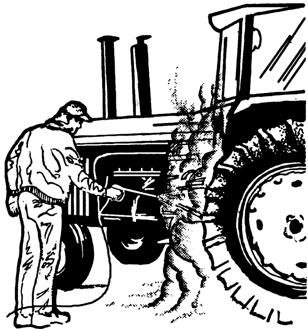
Proper Surface Preparation Begins With Proper Cleaning
